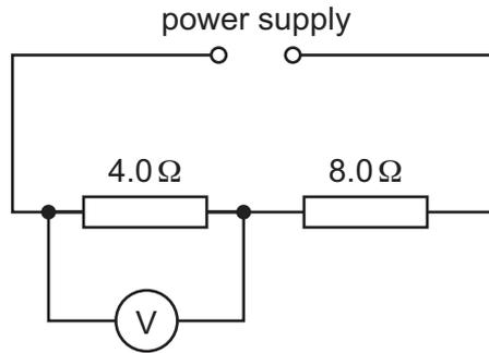
The reading on the voltmeter connected across the  $4.0\ \Omega$  resistor is  $2.0\ \text{V}$ .
